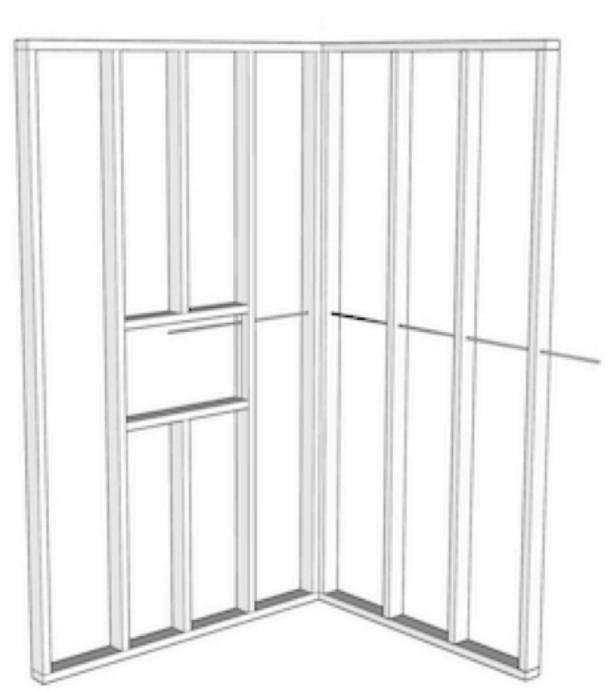
2. Ensure that there is a 1/2"-1" gap between the stud framing and the niche where the low voltage wires will come out. This is so there is adequate room for wire connectors and wire slack to be pulled from in the event there is need to service light channel.
